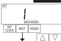
**Step 6CS** – Press the ▼ or ▲ buttons until BACKWASH appears. Press NEXT to go to Step 7CS. Press REGEN to return to previous step.
