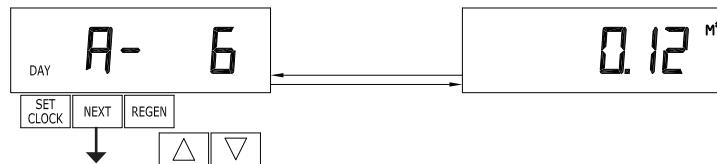
the capacity for days 3, 4, 5 and 6. The **▼** button can be pressed to move backwards in the day series. Press the **NEXT** button at any time to go to Step 5D. Press **REGEN** to return to previous step.
