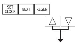
**STEP 1D** – Press **▲** and **▼** simultaneously for three seconds. If screen in step 2D does not appear in 5 seconds the lock on the valve is activated. To unlock press **▼**, **NEXT**, **▲**, and **SET CLOCK** in sequence, then press **▲** and **▼** simultaneously for 3 seconds.
