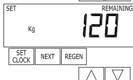
NOTE: Estimate the Kg of salt in the brine tank and add it to the amount of salt added to the brine tank. The example at the left would indicate 100 Kg of salt being added to a brine tank that has 20 Kg remaining.
