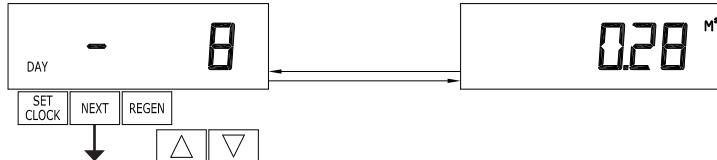
water treated for the last 63 days. If a regeneration occurred on the day the word “REGEN” will also be displayed. This display will show dashes if a water meter is not installed. Press the **NEXT** button at any time to go to Step 6D. Press **REGEN** to return to previous step.
