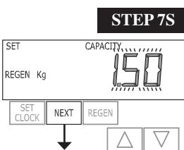
**Step 7S** – Set System Capacity using the ▼ or ▲ button. See chart. The System Capacity setting should be based on the volume of resin and Kg of salt fill set in Step 6S. When using ppm, dH, or FH the system capacity and hardness levels entered are used to determine the Volume Capacity. Press NEXT to go to Step 8S. Press REGEN to return to previous step.
