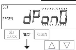
**Step 4CS** – If ALTA or ALTb was not selected in Step 3CS, allows selection of one of the following using the ▲ or ▼ buttons:
