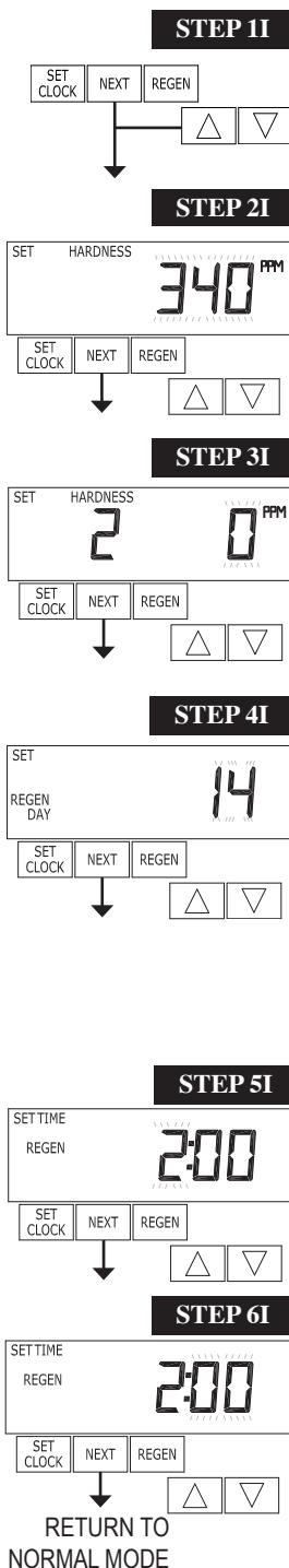
**STEP 1I** - Press NEXT and **▲** simultaneously for 3 seconds.
