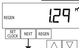
**STEP 3D** – Volume, since last regeneration: This display shows the volume of water that has been treated since the last regeneration. This display will equal zero if a water meter is not installed. Press the **NEXT** button to go to Step 4D. Press **REGEN** to return to previous step.
