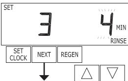
**Step 5S** – Select the time for the third cycle (which in this example is RINSE) using the ▼ or ▲ button. Press NEXT to go to Step 6S. Press REGEN to return to previous step.
