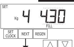
**Step 6S** – Select the Kg or MIN for the fourth cycle (which in this example is FILL) using the ▼ or ▲ button. When both 50 and 50L are options in Step 2CS, and 50 is selected, FILL is in minutes. WS2 valves are shipped from the factory with a refill flow control of 2.2 gpm (8.3 lpm). Press NEXT to go to Step 7S. Press REGEN to return to previous step.
