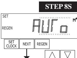
**Step 8S** – Set Volume Capacity using the ▼ or ▲ button. If value is set to:
