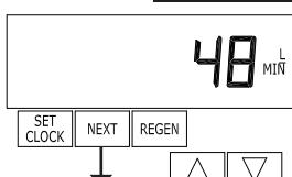
**STEP 6D** – Flow rate, maximum last seven days: The maximum flow rate in liters per minute that occurred in the last seven days will be displayed. This display will equal zero if a water meter is not installed. Press the **NEXT** button to exit Diagnostics. Press **REGEN** to return to previous step.
