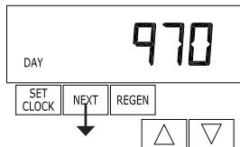
**STEP 2VH<sup>3</sup>** – Days, total since start-up: This display shows the total days since startup. Press the **NEXT** button to go to Step 3VH. Press **REGEN** to return to previous step.
