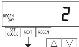
**STEP 2D** – Days, since last regeneration: This display shows the days since the last regeneration occurred. Press the **NEXT** button to go to Step 3D. Press **REGEN** to exit Diagnostics.
