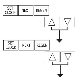
**STEP 1VH** – Press **▲** and **▼** simultaneously for three seconds and release. Then press **▲** and **▼** simultaneously and release. If screen in step 2VH does not appear in 5 seconds the lock on the valve is activated. To unlock press **▼**, **NEXT**, **▲**, and **SET CLOCK** in sequence, then press **▲** and **▼** simultaneously for 3 seconds and release. Then press **▲** and **▼** simultaneously and release.
