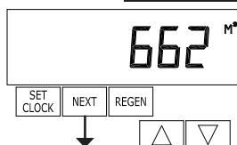
**STEP 4VH** – Volume, total used since start-up: This display shows the total volume of water treated since startup. This display will equal zero if a water meter is not installed. Press the **NEXT** button to go to Step 5VH. Press **REGEN** to return to previous step.
