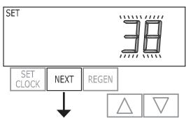
**Step 2CS** – Use the ▲ or ▼ to select 25 for WS1 valve, 32 for WS1.25 valve, 38 for WS1.5 valve, 50 for WS2 or 50L for a WS2L valve.<sup>1</sup> When 50 or 50L is selected, an additional screen will appear. It is used to select which size flowmeter is to be used with the valve, 38mm or 50mm. Press NEXT to go to Step 3CS. Press REGEN to exit OEM cycle sequence.
